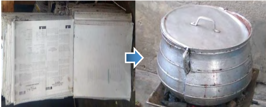
Figure 5: Used offset plate converted into metal cooking pots to reduce environmental impact
