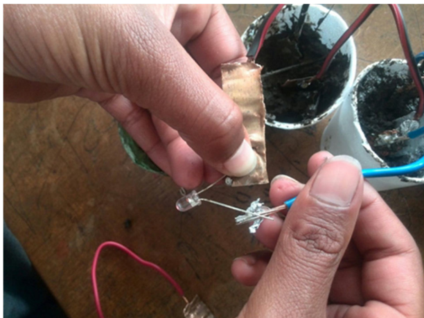
Figure 2 : Current produced from microbial fuel cell could light up an LED
