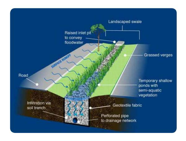
Figure 8: Schematic of a typical bioswale system (FAWB, 2009:5)
